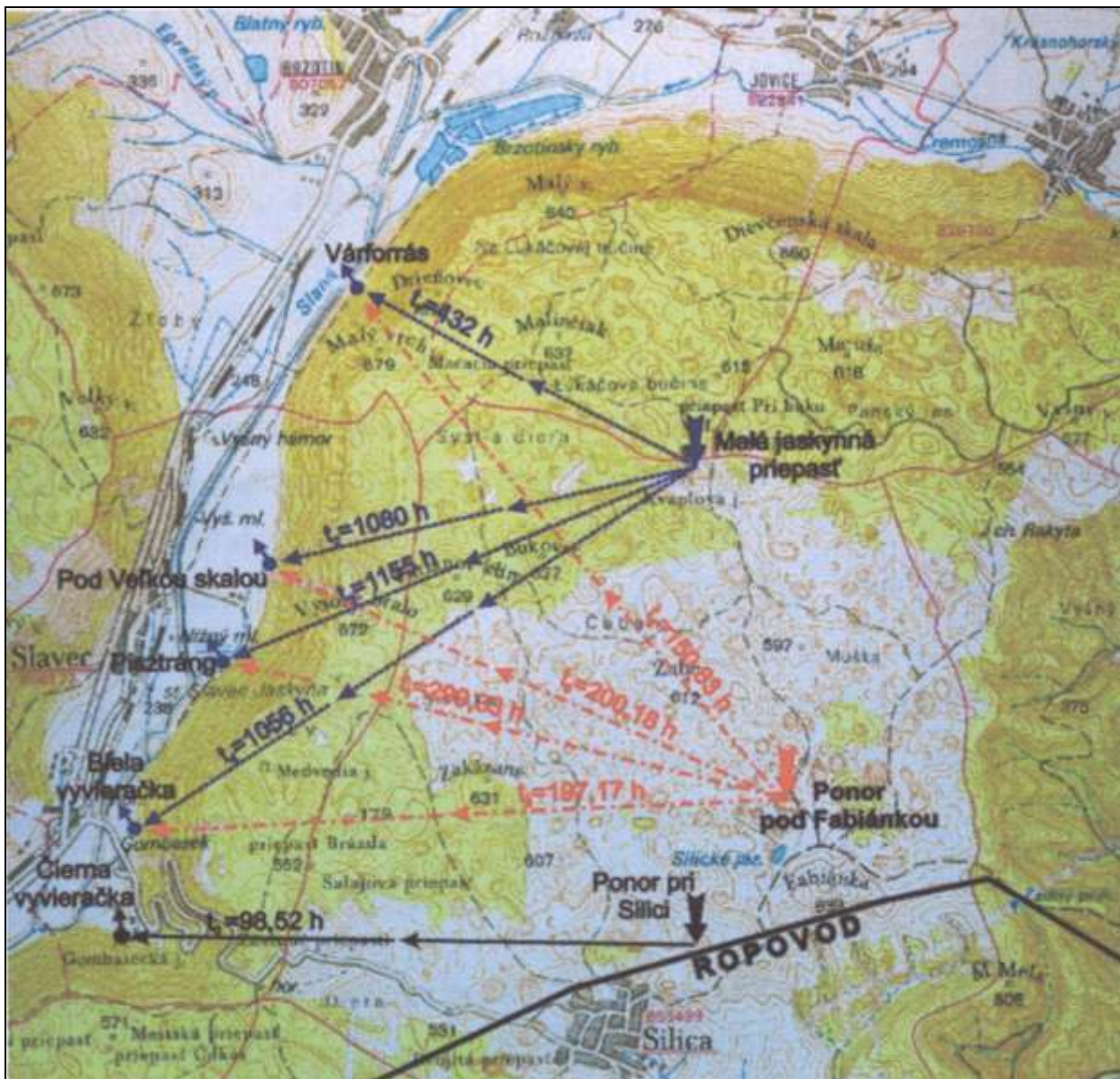
Fig. 4.1.16 Water connections of the Silica Plateau in the surroundings of the “Friendship” oil pipe (ropovod)
