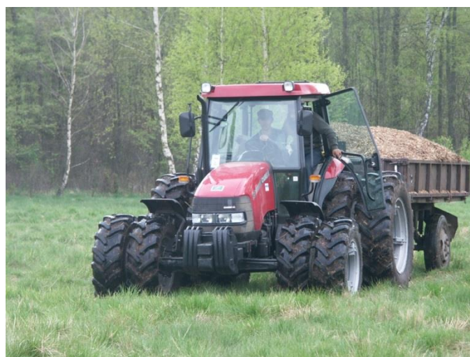
Woodchip removal using tractor with double tires for working on wet areas © CMOK archive
